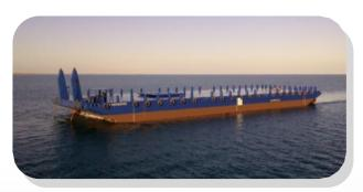
A.M.S. HENDERSON 250ft x 80ft x 16ft Deck Cargo Ballast Tank Barge
